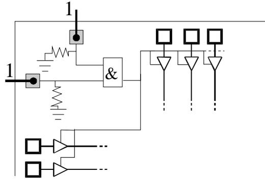
**Figure 2. Automatic selection of pad cells**
