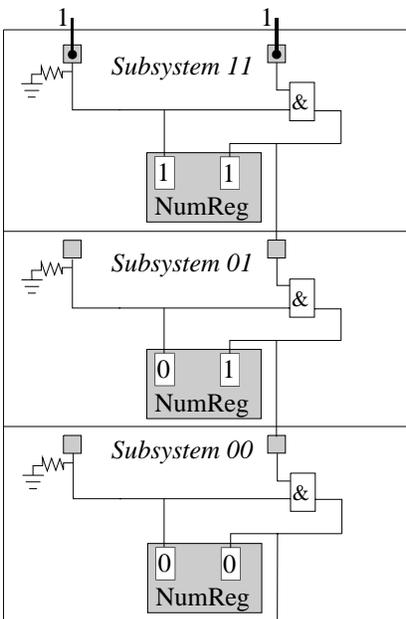
**Figure 3. Circuitry for numbering of *AxPe-Subsystems***
