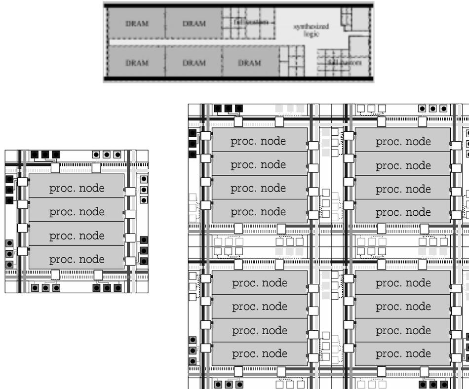
**Figure 1. Floorplan of processing node (PN) (top), *AxPe-Subsystem* (left bottom) and *AxPe-LAIC* (right bottom)**
