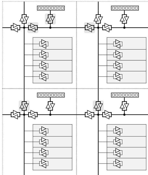
**Figure 5. Schematic representation of in-out bus with bi-directional repeaters**
