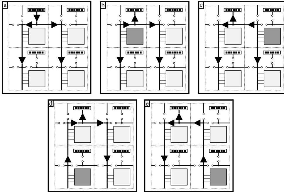
**Figure 4. Signal flow of bi-directional bus system with host-IC as source (a) and different subsystems as source ((b) to (e))**
